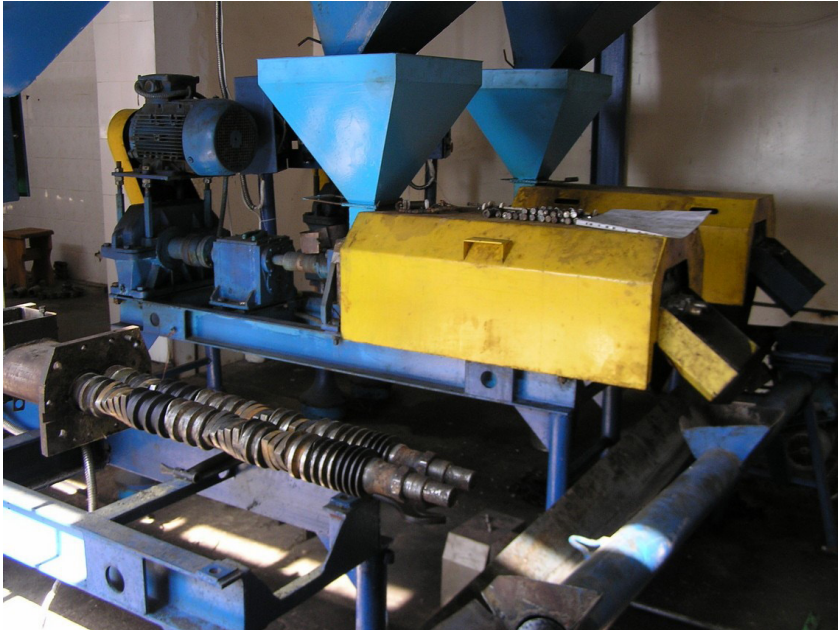
Figure 4. General view of experimental extrusion presses EK 75/1200
