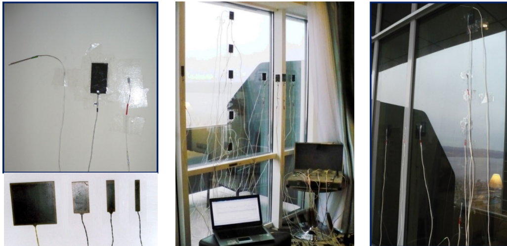
Figure 3. Measuring sensors of various modifications (a) and their installation during field tests on the inner surface – heat flux sensors (b); on the outer surface – temperature sensors (c)
